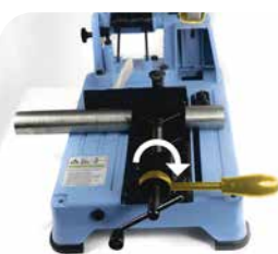
5. Turn the lever to the right and start the sawing process: next steps: 3 - 4 - 5.
