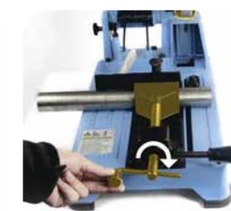
2. The material to be sawn is fixed with the spindle (one-time process).
