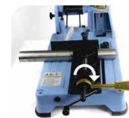
1. Starting position: The quick release lever is on the right.
