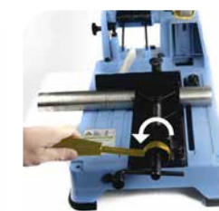
3. After the cut, the quick release lever is placed on the left side.
