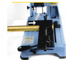
4. The next workpiece is brought into the position to be sawed.
