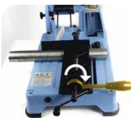
5. Turn the lever to the right and start the cutting process: next steps: 3 - 4 - 5.
