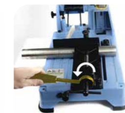
3. After the cut, the quick release lever is placed on the left side.
