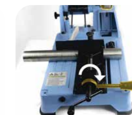
5. Turn the lever to the right and start the cutting process: next steps: 3 - 4 - 5.
