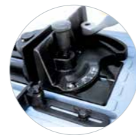
MITER CUTS CAN BE ADJUSTED WITHOUT TOOLS 90-75-60-45°
