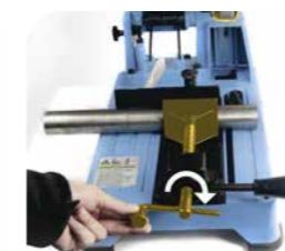
2. The material to be sawn is fixed with the spindle (one-time process).
