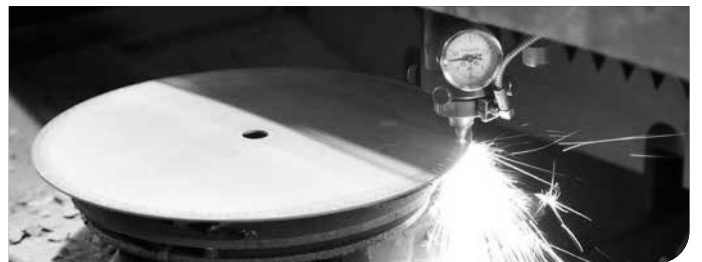
lasering the segments
