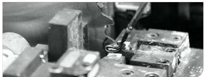
soldering the carbide teeth
