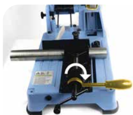
1. Starting position: The quick release lever is on the right.
