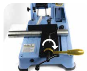
5. Turn the lever to the right and start the cutting process: next steps: 3 - 4 - 5.
