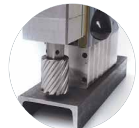
Core drilling up to \varnothing 52 mm
