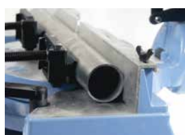
Fixation set „K“ for tubes Ø 30 mm up to 70 mm
