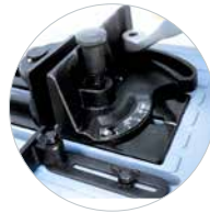
MITER CUTS CAN BE ADJUSTED WITHOUT TOOLS 90-75-60-45°
