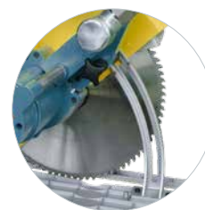
Depth adjustment with scaling
