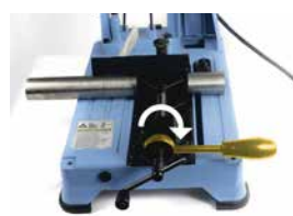
Vice with quick release system for series cut
