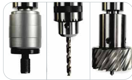
Thread cutting, twist- & core drilling (accessories might be necessary)
